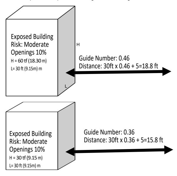
The burning building is called the exposing building, while the other which is threatened is called the exposed building.
